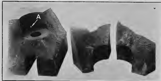
FIG. 5. HIGH-SPEED STEEL DIE BURST BY RAPID GENERATION OF STEAM
